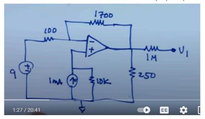
a) What is the relationship between the inverting terminal and the non-inverting terminal
